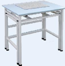
Anti-vibration table designed mainly for industrial scales. A steel construction with an MDF top and a stone stabilizing plate placed on an independent footing.
