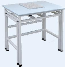
Anti-vibration table for analytical, laboratory and controlling balances. A steel construction with an MDF top and a stone stabilizing plate placed on an independent footing.
