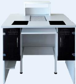
A weighing station for microbalances and analytical balances also used as a workstation for pipettes calibration. A steel construction of the anti-vibration table with a stone top is enclosed in an elegant desk layout made of MDF.
